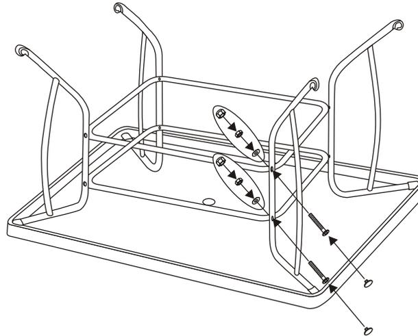
**Step 4:** Tighten all nuts and bolts using the Hex Bolt Driver and Hex Wrench provided. Important note: each bolt should be tightened a few revolutions at a time, alternating between bolts in a cross corner ("X") fashion. This will ensure your table is level by placing equal pressure on all bolt joints. Do not over tighten. Cover all nuts and bolts with PVC covers provided.
