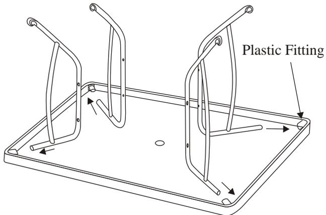
**Step 3:** Attach leg connector bracket (begin with the leg connector bracket closest to the table) by inserting bolt through the table leg and leg connector bracket. Secure bolt with nut. **Hand tighten only** (do not fully tighten bolts at this time as some adjustments may be necessary between the leg connector bracket and the legs to ensure proper alignment of the table legs). Repeat for remaining table legs. Repeat procedure for remaining leg connector bracket.
